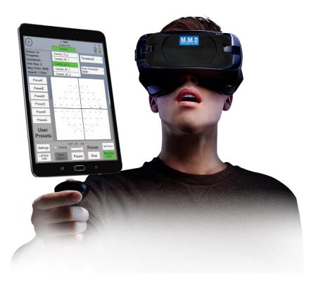
PalmScan VF2000 is a portable, battery operated, virtual reality based visual field analyser, developed to be able to measure the patient visual field defect accurately, and reliably. The VF2000 is composed of 3 major sections that are connected to each other wirelessly and there are no wires to deal with when using this system. The 3 major components are:<sup>[4]</sup>
